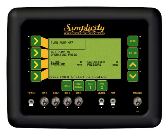
**Calibrate Pressure Sensor Screen**
