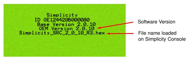
The above screen is displayed for 60 seconds each time the Simplicity Console is switched ON, using the 'POWER', button.
