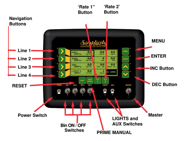
**RESET -** The RESET button allows the bins to be refilled in the console when the bins are empty. (See Section 7.1 for details).
