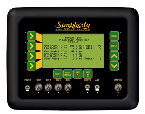
**Sensor Test Screen (Hydraulic)**
