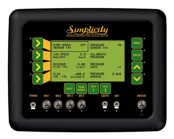
Liquid Tank Setup '2' Screen (with Pressure Sensor 'ON')
